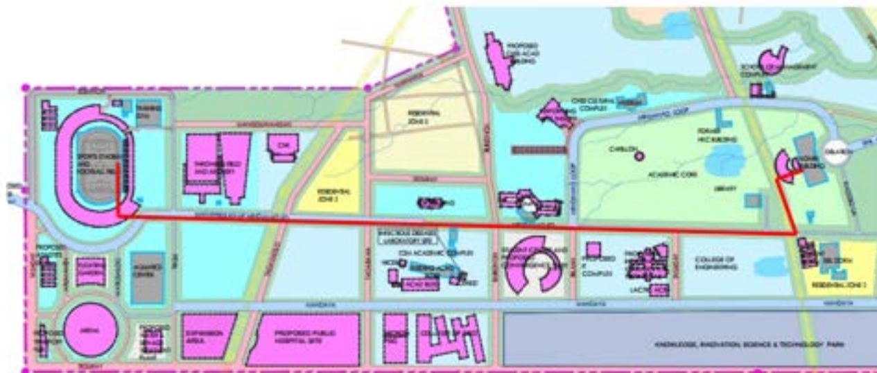
12 -CORE FOC SM Aerial installation Using existing poles
